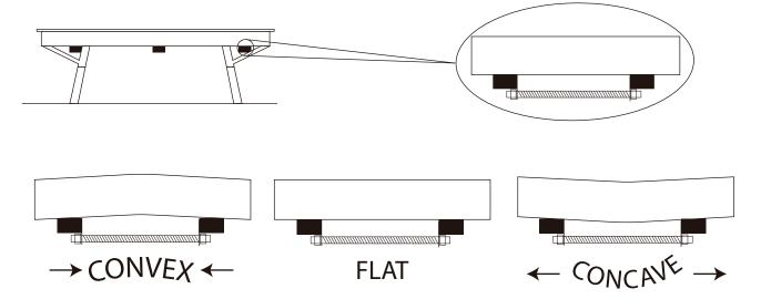
NOTE: Adjusting the Bolts inward will make the planks convex. Adjusting the Bolts outward will make the planks concave.
